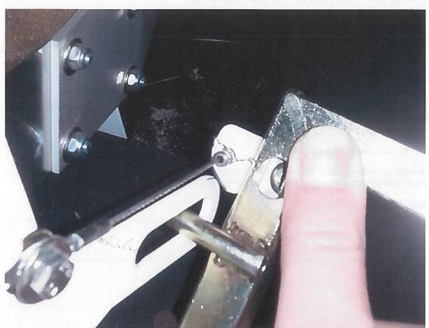
Fig 1. Throttle cable bracket (top right) modified with bottom corner cut off to miss throttle stop plate (on the left). Note wirelocking of throttle ferrule.
